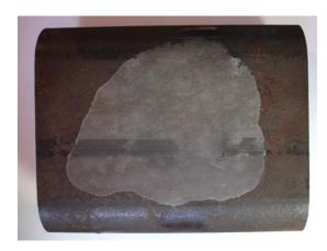
• Remove any remaining solution with a cloth or water. Try to remove the rust when the gel is still wet.
