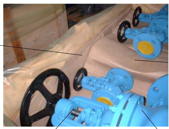
Corrugated cardboard separators used as cushioning can be a significant source of corrosion.
