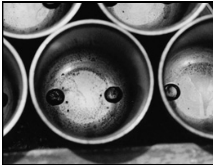
Figure 2b: Closeup of MILES tubes with signs of powder residue and corrosion. With a recovery time of 30 minutes for four Hoffmans, there are less troops needed to clean the Devices using Evapo-Rust.
